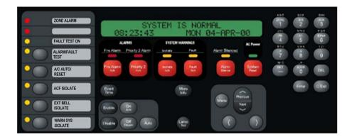
Figure 2-3. Operator Interface
